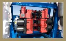
Hydraulically operated floor hand makes and breaks drill rod and collars in an extremely safe manner. Unit retracts to back of derrick to provide easy clearance of the drill string.
