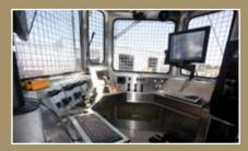
Driller's cabin is climate-controlled with enhanced electric over hydraulic controls for all rig functions. Monitors capture all drilling parameters from two remote-cameras. Information can be viewed via the internet.
