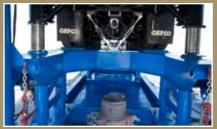
Telescoping substructure allows for ten-foot standard clearance between ground level and bottom of the table. Rig uses hydraulic leveling jacks which are mechanically locked for safety.
