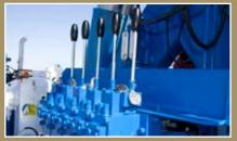
All electronic controls feature manual backup controls to give the operator redundancy in case of an electrical failure.
