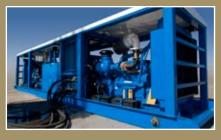
1100 HPU separate power pack is remotecontrolled and powered by two 550 hp CAT C-18 engines. One engine can operate all rig functions. Unit is connected through a series of quick-connected hydraulic hoses.
