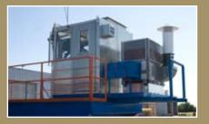
Cabin is equipped with a climate-controlled fresh-air purge system so it meets Class I Division I explosion-proof standards.
