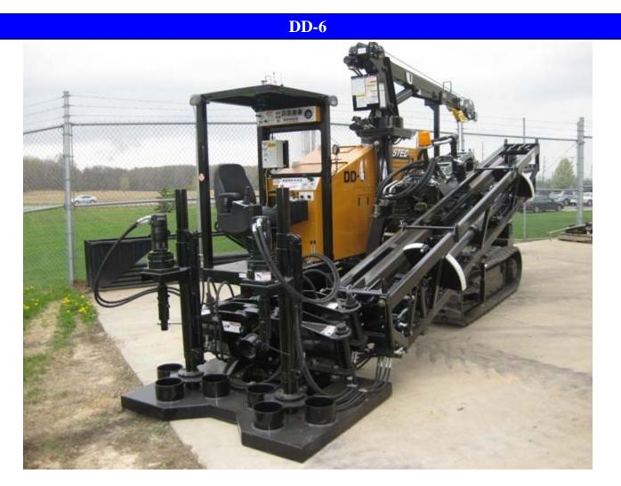
The ASTEC® branded DD-6 is a self-contained horizontal directional drilling system. The DD-6 allows contractors to utilize its compact size to operate in urban, suburban, and other hard-to-reach jobsites. The DD-6 incorporates rugged construction, a field-proven design, and mechanical fortitude that makes this machine an ideal mid-size HDD solution when facing the toughest of trenchless jobs.
